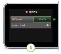
Hold the pump and tubing vertically to ensure any air in the cartridge will be pushed out first. Tap **START.** The pump will beep or vibrate regularly while the tubing is filled.
