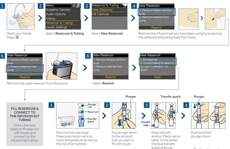
**Warning:** Do not use the reservoir or infusion set if any liquid gets on the top of the reservoir or inside the tubing connector. Liquid can temporarily block the vents and may result in the delivery of too little or too much insulin, which can cause hypoglycemia or hyperglycemia.
