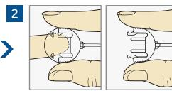
Press the edges of the set release connector. With the other hand, pull the cap off.
