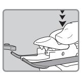
2. Place Silhouette<sup>®</sup> insertion piece inside Sil-serter<sup>®</sup> and let go of the Lock & Release handle. The serter should fit securely into the holes of the insertion piece.
