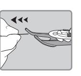
Hold Silhouette<sup>®</sup> in place against skin with one hand. With the other hand press Lock & Release handle using thumb to open serter. Then, slide serter back from Silhouette<sup>®</sup>.
