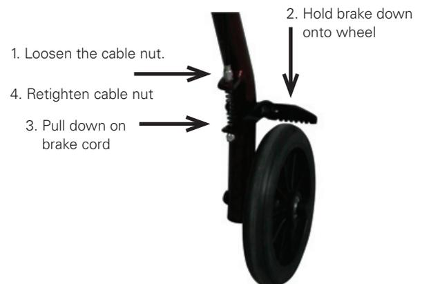
**Caution:** After making any adjustments to the rollator brakes, you must test the brakes before the rollator is used. See Maintenance instructions.
