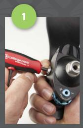
Remove the 4 mm axial pin
