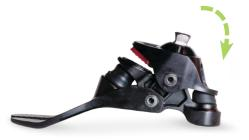
On heel strike, the rear bumper compresses to bring the toe down to foot flat. This gives higher rates of ground contact on declines for firm footing.
